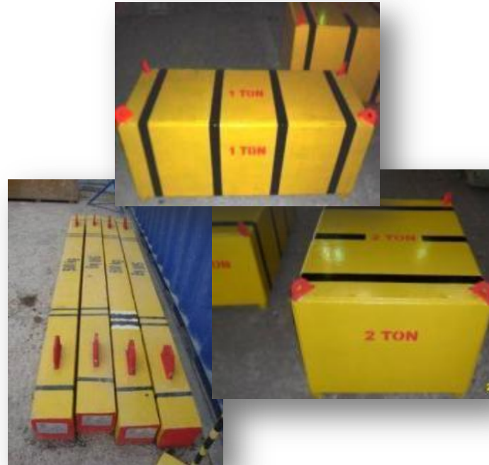
Load Test Weights
